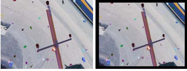
Fig. 3. Visualization of the homography mapping between two different camera parameters. Note, the original sizes of the images are 1280 x 960 and 640x480, respectively for the left and right image.
