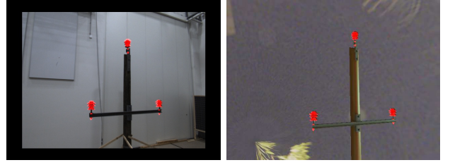
Fig. 4. Reprojection of the 6-DoF object poses predicted by PoET (TRT Small FP16) for our real-world scenario (left) and a synthetic image (right). Note that the black border for the real image is due to the homography mapping between different camera parameters.
